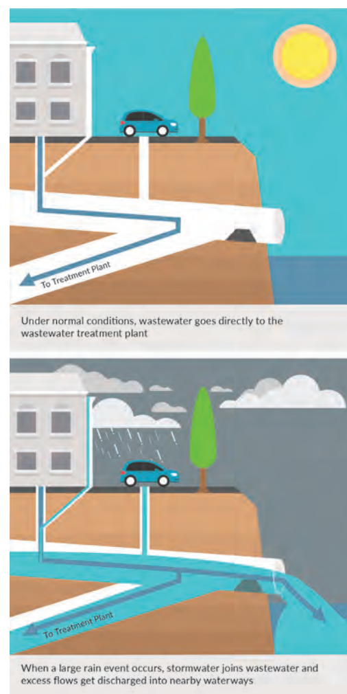
Figure 3 A typical combined system
