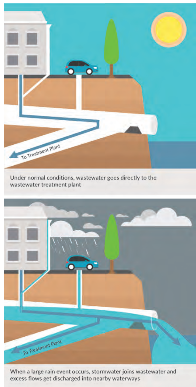
Figure 3 A typical combined system
