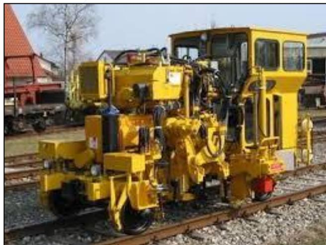
Figure 5. – Example of a small tamping machine
