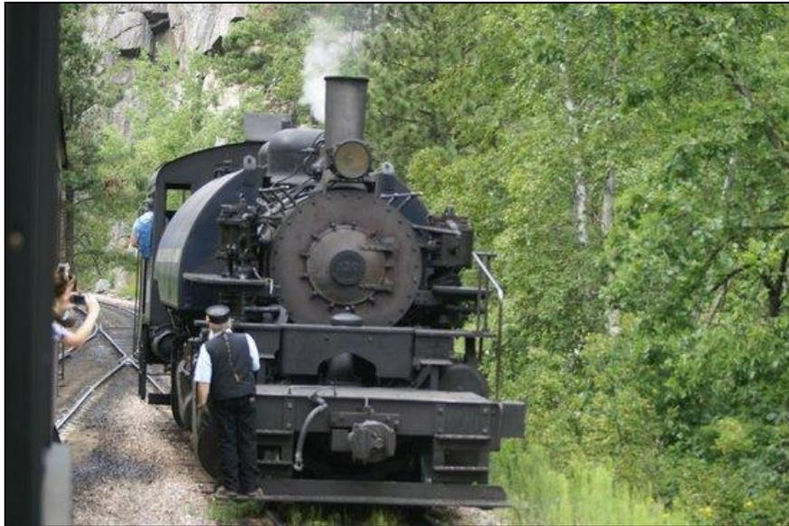
Figure 23. – A steam loco changing ends on a typical engine run around track
